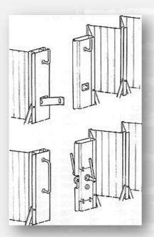
For concrete lintels 1/2"BSW through or rag bolts with 38mm thread projection should be supplied and fitted by you. For steel work we will generally require 14mm dia holes by others, however we shall be pleased to advise further upon receipt of your opening details.
