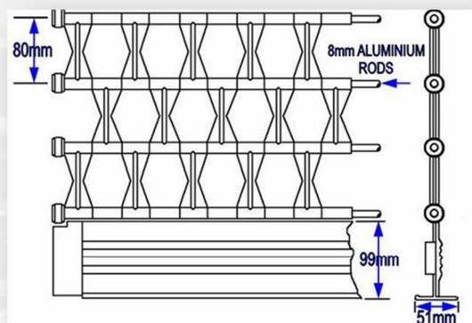
Constructed from high quality injection moulded plastic links assembled on 8mm diameter heat treated alloy rods, the plastic grille has 22mm diameter nylon end guides fitted to each end of every rod to facilitate ease of movement. The nylon guides are in lipped side channels designed to prevent the grille curtain from being forcibly removed and help deter unauthorised entry. Plastic links are produced in five standard colours, white, black, grey, red and brown.
